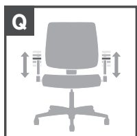
Q. Adjustable height arms — Provide improved upper-torso support. Can be adjusted periodically to relieve strain and provide variety.
