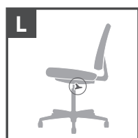
L. Tilt lock — Locks out tilt function.
