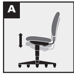
A. Pneumatic seat height adjustment — Regulates height of chair relative to floor.
