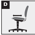
D. Seat glide mechanism — Seat cushion travels forward and back, then locks into position.
