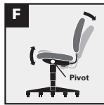
F. Tilt — Pivot point located directly above center of chair base.
