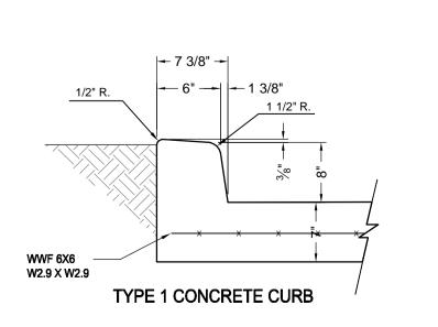
INTEGRAL CONCRETE CURBING DETAIL
