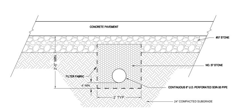
FREE DRAINING BASE TRENCH & PIPING DETAIL C2-2 NO SCALE:
