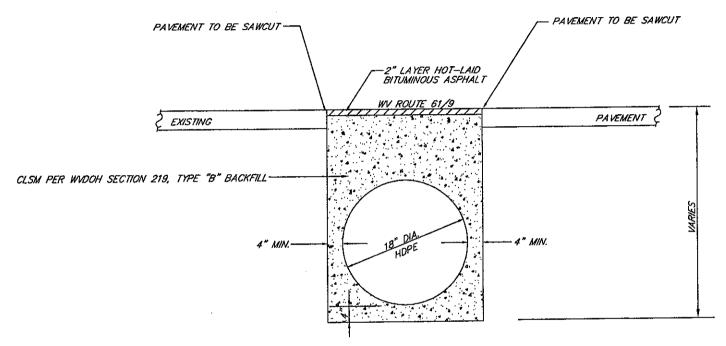
NOTE: ANCHOR PIPE SO TO PREVENT FLOATING DURING BACKFILLING OPERATIONS.
