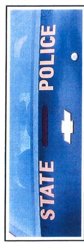
GRAPHIC FOR "STATE" WILL BE DIE-CUT 3M SERIES 690 REFLECTIVE, REMOVABLE SHEETING, GOLD 690-64 OR EQUAL. LETTERING WILL BE A MINIMUM OF 2 \*\*116\*\*\* IN HEIGHT, WITH THE WORD "STATE" MEASURING MINIMUM OF 9 \*\*116\*\* AND MAXIMUM OF 9 \*\*116\*\*\* AND MAXIMUM OF 9 \*\*116\*\*\* AND MAXIMUM OF 9 \*\*116\*\*\* IN LENGTH.
