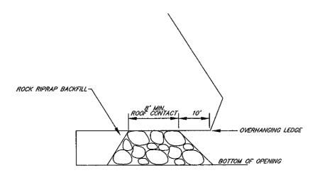
NOTE: BACKFILL FULL LENGTH OF OVERHANGING LEDGE
