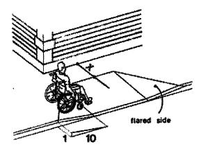
Note: If X is less than 48 inches, then the slope of the flared side shall not exceed 1:12. This figure shows a typical curb ramp, cut into a walkway perpendicular to the curb face, with flared sides having a maximum slope of 1:10. The landing at the top, measured from the top of the ramp to the edge of the walkway or closest obstruction is denoted as "x". If x, the landing depth at the top of a curb ramp, is less than 48 inches, then the slope of the flared side shall not exceed 1:12.
