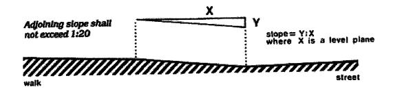
The ramp slope is a ratio equal to the vertical rise (y) divided by the horizontal run (x). It is equal to the tangent of the angle that the plane of the ramp surface makes with a horizontal (level) plane. For a curb ramp, the adjoining slope at walk or street shall not exceed 1:20.
