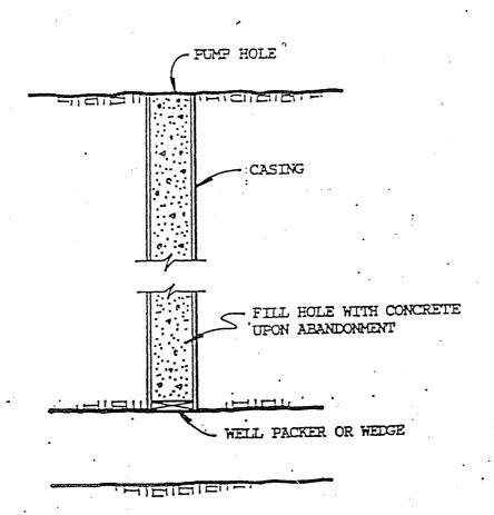
TYPICAL DETAIL BORE HOLE SEAL (not to scale)
