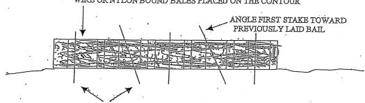
2-2 INCH X2 INCH-STAKES, 1 % FEET TO 2 FEET IN THE GROUND
