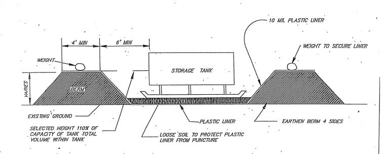
Note:  $\Lambda$  2" water removal drain shall be located at the lowest point in the bottom of the containment volume. It shall connect to a normally closed gate-valve outside the dike. The gate valve is manually operated and protected from unauthorized operation. Rainwater contained within this dike shall be examined prior to release to ensure that harmful quantities of fuels and lubricants are not discharged.
