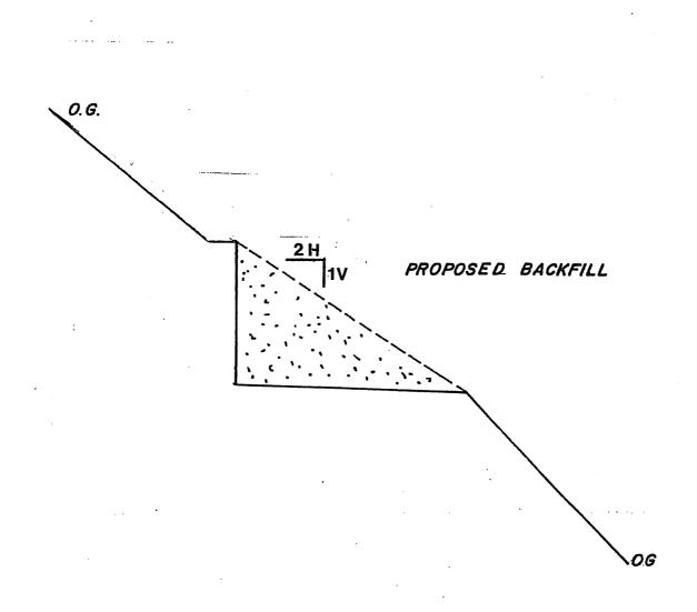
REGRADE X-SECTION LOADOUT
