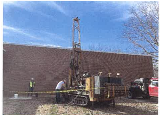
Investigation of the subsurface conditions with standard penetration test borings at the Tidewater Community College campus
