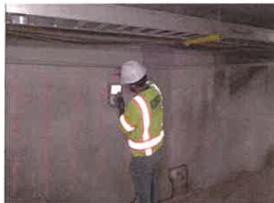
Surface Penetrating Radar to locate embedded reinforcement
