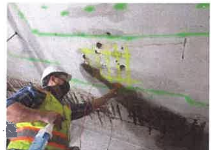
Half-cell testing for reinforcing steel corrosion
