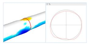
Our main-sewer inspection cameras have other talents, too: Equipped with an optionally available scanning function, they detect even the smallest deformations in main lines using 2-point precision lasers and measure them precisely – both point by point and across the entire reach. Due to the 3D display of the pipe, deformations can be determined perfectly.
