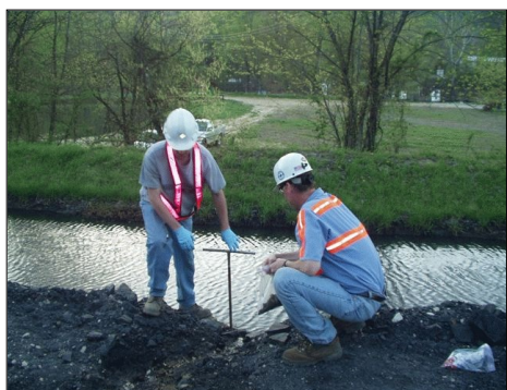
Soil Sampling - Hand Auger
