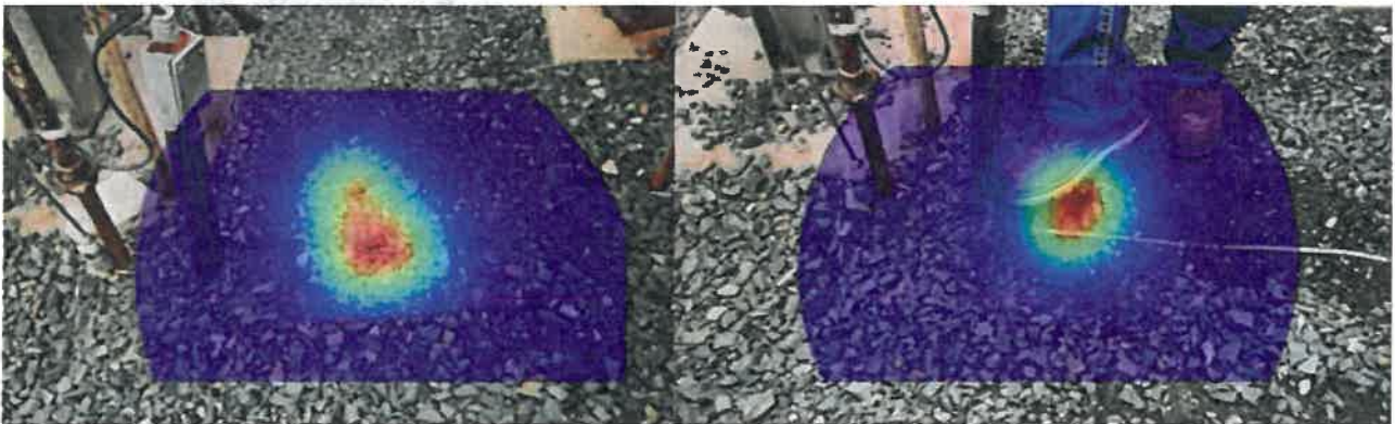
Figure 36. Emission detected under gravel and recorded on a tubing after removing gravel.
