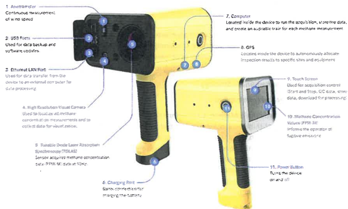
Figure 1. Xplorobot Laser OGI device and its elements
