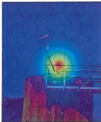
Figure 11. Visualization of emission is otherwise not visible to the naked eye, attributing the emission to the specific components (bolt, thief hatch) and detection of emission from an underground pipe.
