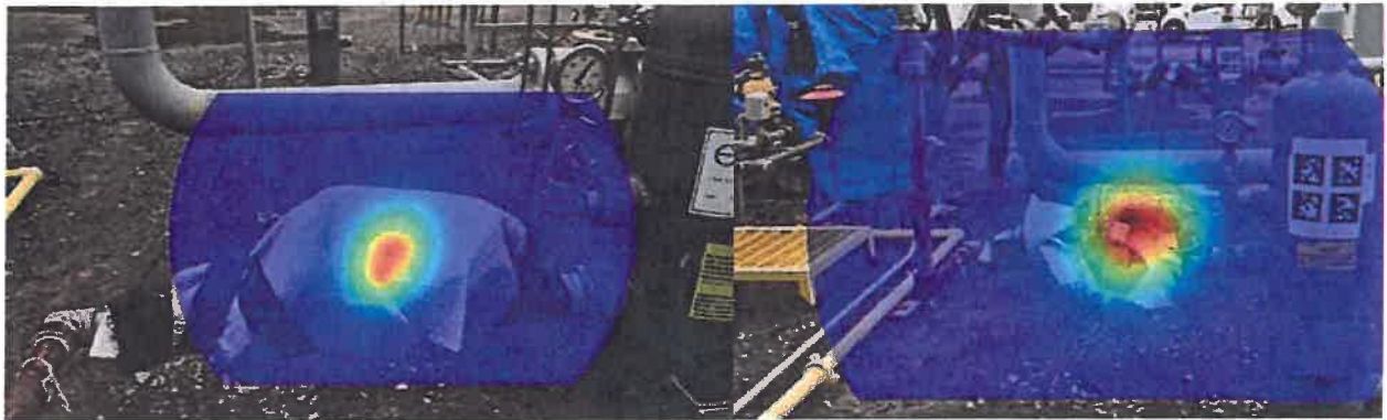
Figure 20. Emissions were detected under a bubble wrap, and the recording on the regulator after the wrap was removed.
