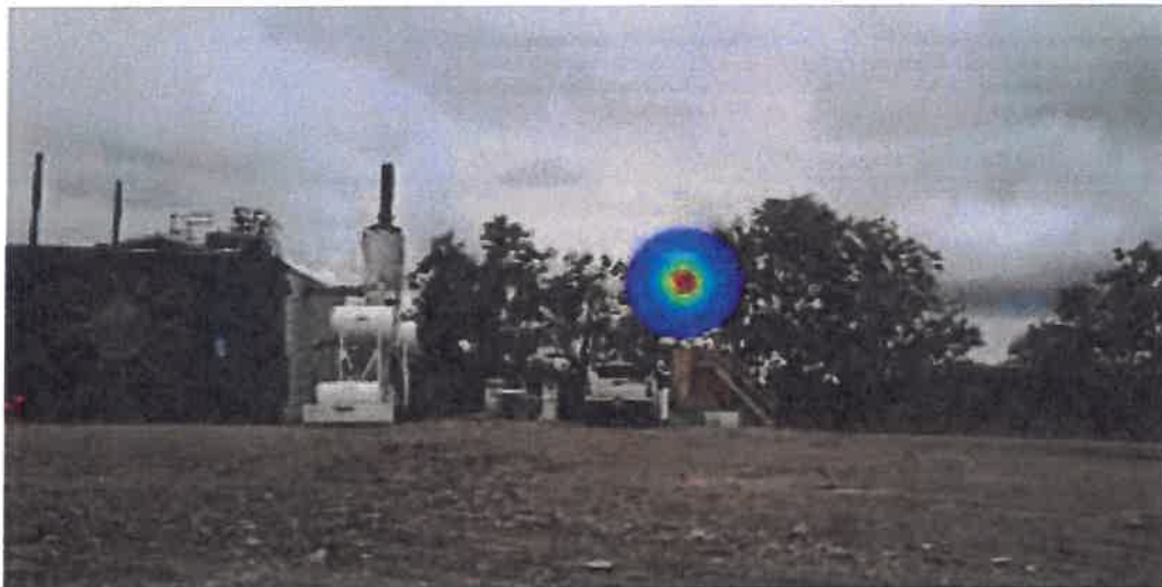
Figure 14. Detection of an open vent emission utilizing the tree behind the vent to reflect the laser.
