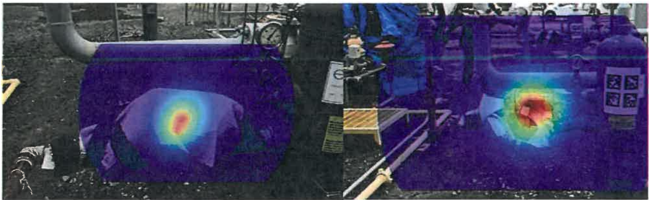
Figure 35. Emissions detected under a bubble wrap and the recording on the regulator after the wrap was removed.
