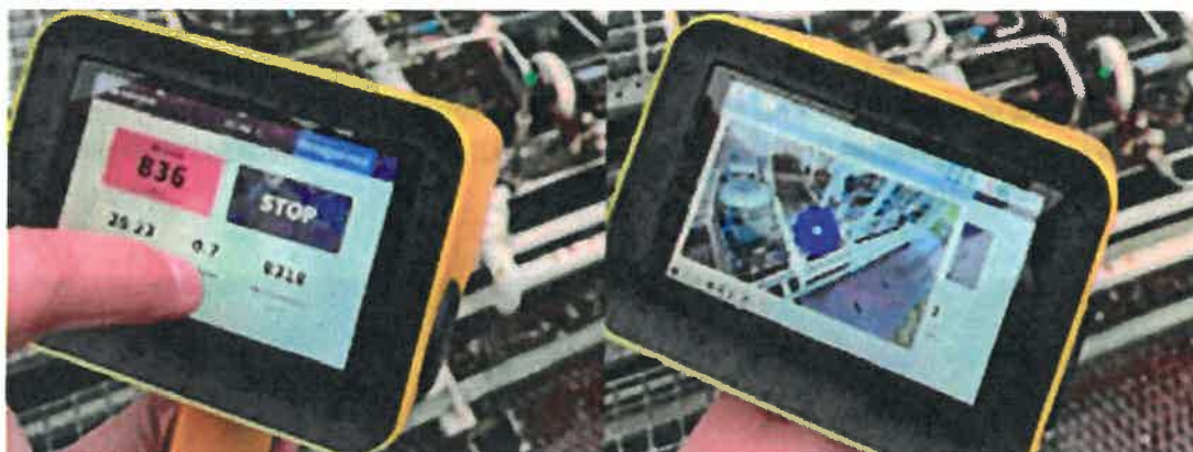
Figure 7. Visualization of methane emission is otherwise not visible to the naked eye, attributing the emission to the specific component (flange).
