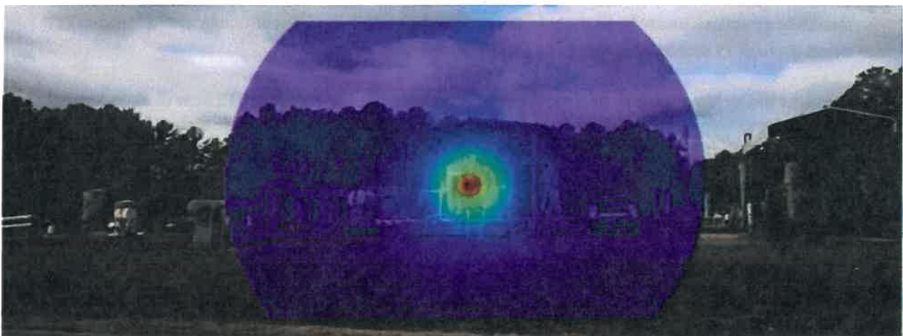
Figure 37. Emissions detection from outside the plant gates across the road.
