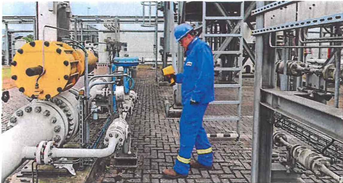
Figure 10. Scanning equipment and components with Xplorobot Laser OGI device.
