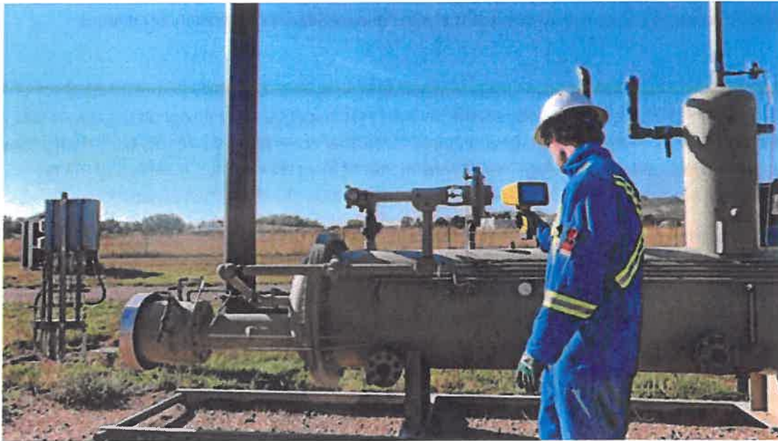
Figure 39. A person without LDAR certification or any special training successfully operating Xplorobot Laser OGI scanning a separator in METEC, Fort Collins, Colorado.
