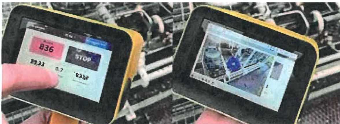
Figure 10. Detection of the emission (concentration above 500ppm-m) and visualization of the emission otherwise not visible to the naked eye by the Xplorobot Laser OGI device.
