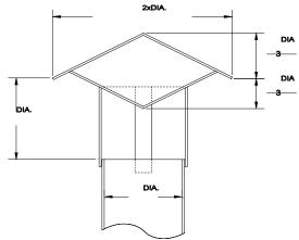
FIG. 1.8.12B: LOW RESISTANCE VENT CAP
