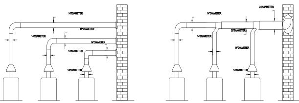
FIG. 1.8.14: SUGGESTED APPLIANCE VENTING PROCEDURE
