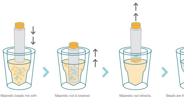
Beads are then released by moving the magnetic rods out of the tip comb; tip comb also facilitates the mixing of reagents with the beads as the magnetic head moves up and down
