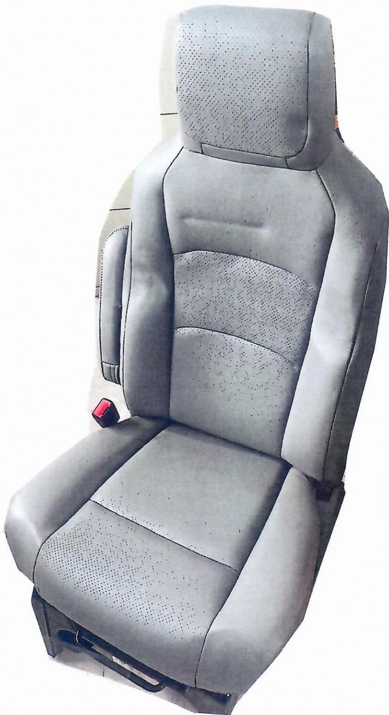
Ford OEM cloth seat mounted on Freedman Adnik power seat base
