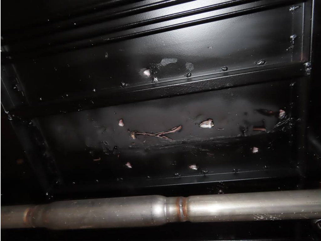
SCRAPES AND GOUGES ON UNDERSIDE OF BUS
