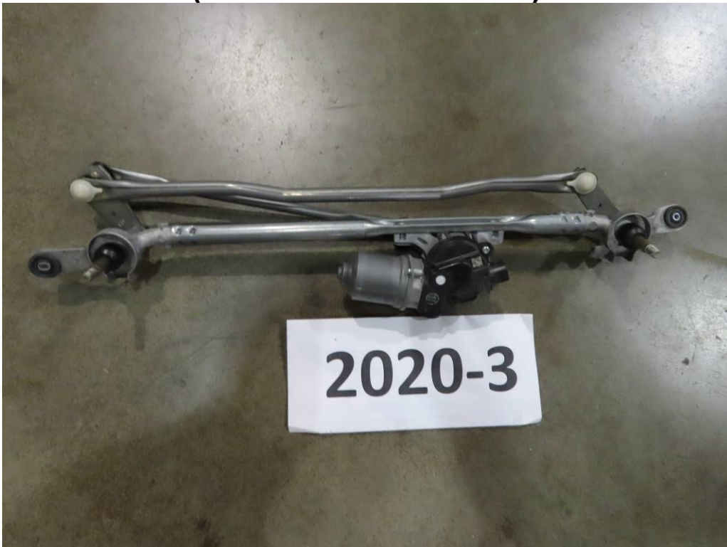
WIPER MOTOR REMOVAL AND REPLACEMENT (0.50 LABOR HOURS)
