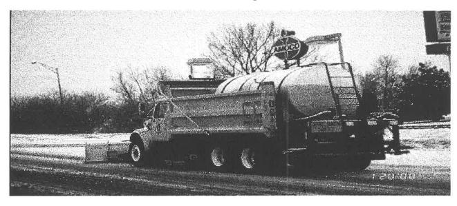
Apply before storm event to prevent Bonding Apply at 30-40 gals / Ln mile\*\* Reduced application rates 30% Reduce application rate for Frost protection - bridges Residual will last 4-6 days
