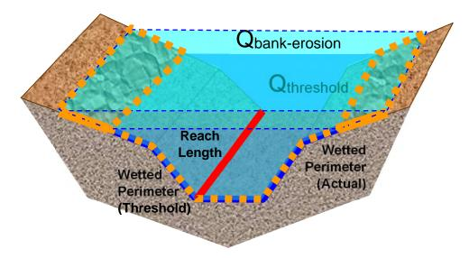
Figure II.B-5. Conceptual diagram of bank erosion model
