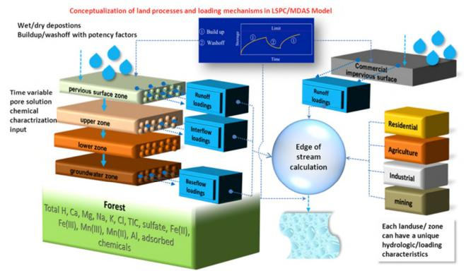
Figure II.B-2. Land components of LSPC-MDAS model
