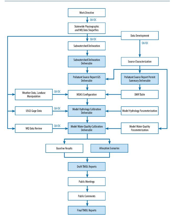
Figure II.G-1. TMDL Development Process Flowchart
