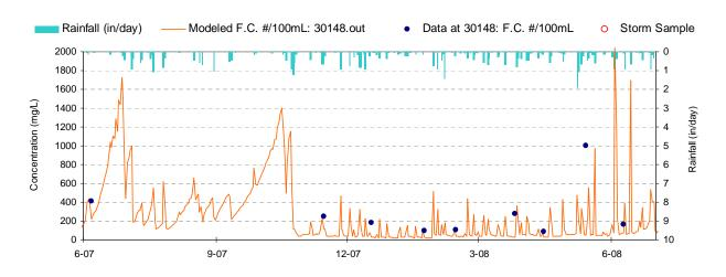
Figure II.B-7. Fecal coliform concentration: model output vs. observed data
