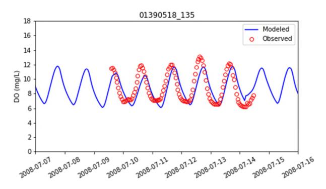
Figure II.B-8. Dissolved Oxygen concentration: model output vs. observed data
