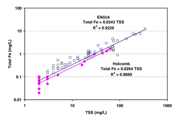
Figure II.B-4. Metals-sediment correlation
