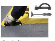
Use a Linea Groover to create the groove between logo and main material. You may use our Triangular Groover to refine the groove.
