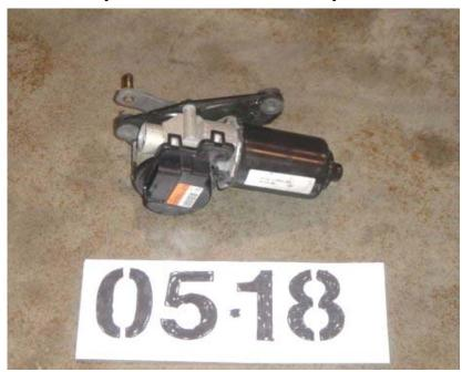
WIPER MOTOR REMOVAL AND REPLACEMENT (0.50 MAN HOURS)
