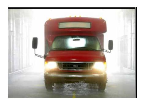
The motorized vehicle rain booth adds front wall nozzles to the design of the towable rain booth, simulating the pelting of oncoming rain at highway speeds. Both booths include two 1200 gallon recycling tanks and utilize a 12Horsepower pump with multi-bank filters capable of delivering 40 – 60 p.s.i. That equates to 300 gallons per minute pushed through the spray heads, or the equivalent of a 24 inchper-hour downpour!
