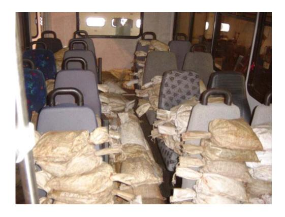
DIAL INDICATORS IN POSITION BUS LOADED TO 2.5 TIMES GVL (10,725 LBS)
