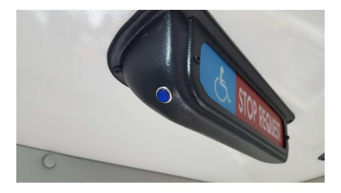
The ADA Occupant Stop Request Lights the Blue Side of the Sign and Signals Driver of an ADA Stop Request via Touch Tape Switches.
