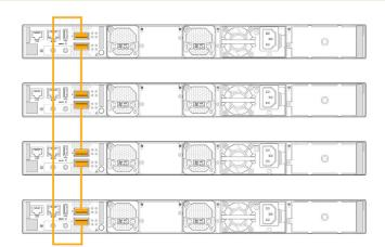
Figure 1: EX4400 Virtual Chassis configuration interconnected via dedicated rear-panel 100GbE ports
