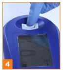
Use only completely filled cuvettes for measuring. A filled cuvette should be analyzed within 1 minute after filling. A filled cuvette should be kept in a horizontal position until measurement.
