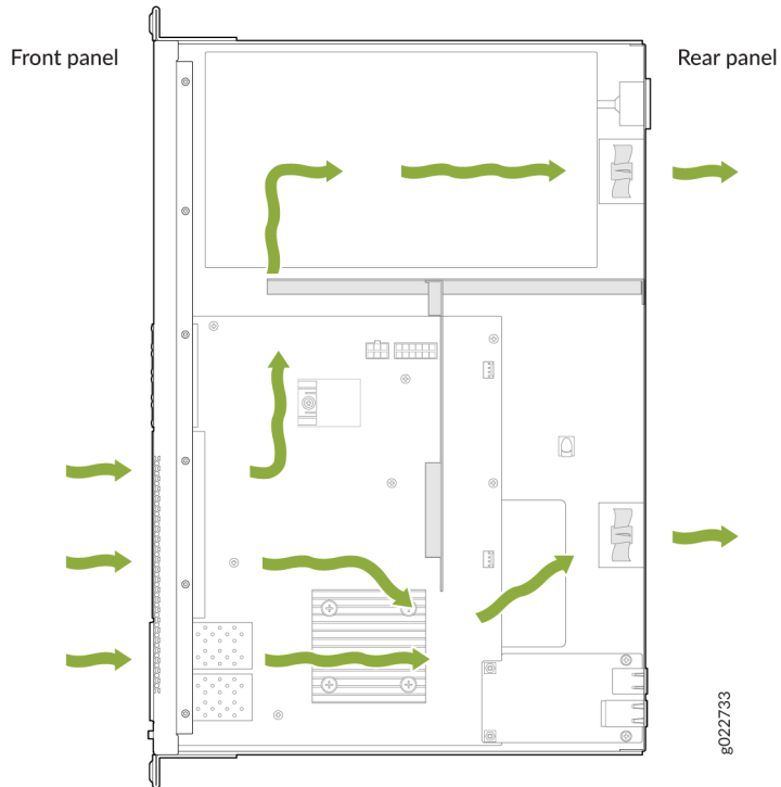
Figure 47: Front-to-Back Airflow Through the EX4100-F-24P Switch Chassis
