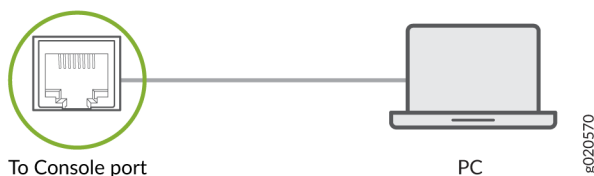
Figure 96: Connect a Device Directly to a Management Console
