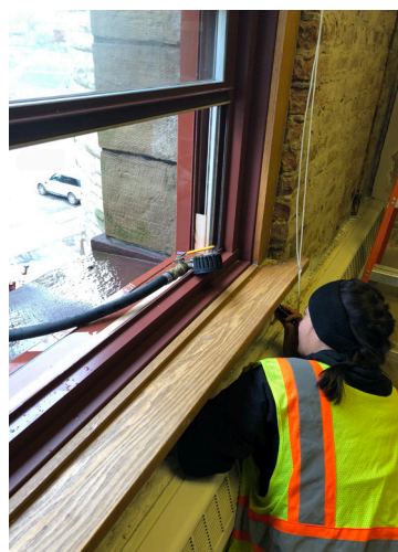
SGH performed water testing at second floor windows.
