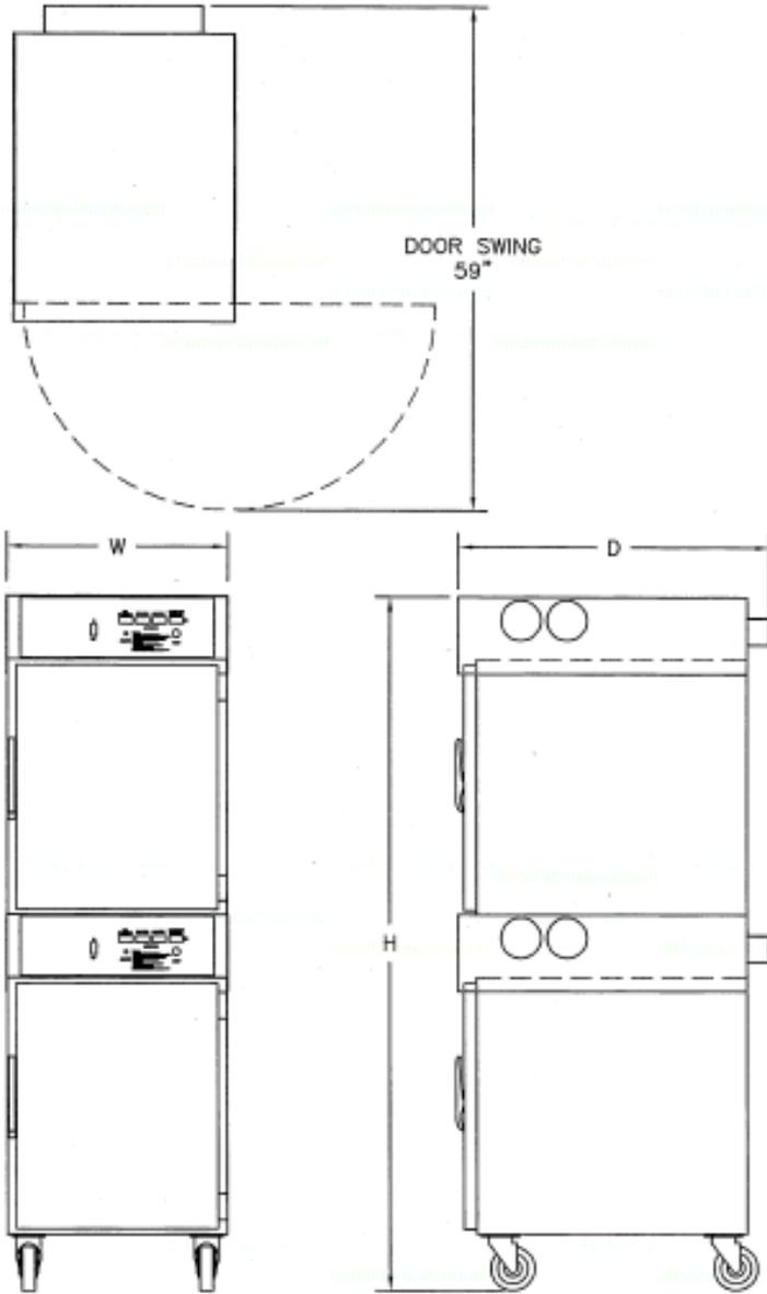
Allow 4" of clearance on each side for ventilation.
