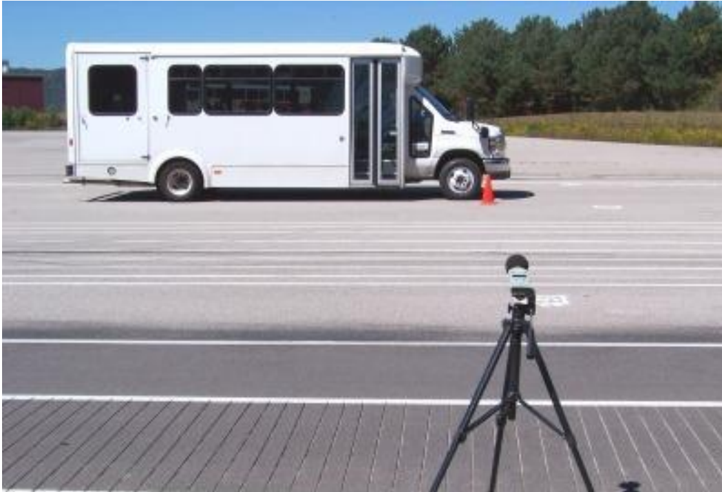
TEST BUS UNDERGOING EXTERIOR NOISE TESTING
