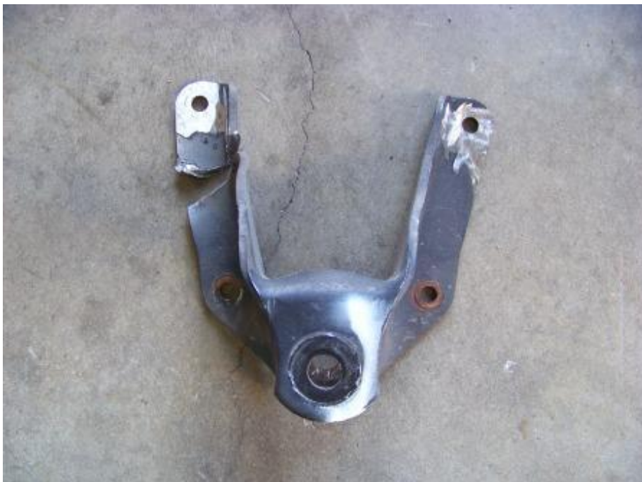
BROKEN RIGHT REAR SPRING HANGER (3,071 TEST MILES)
