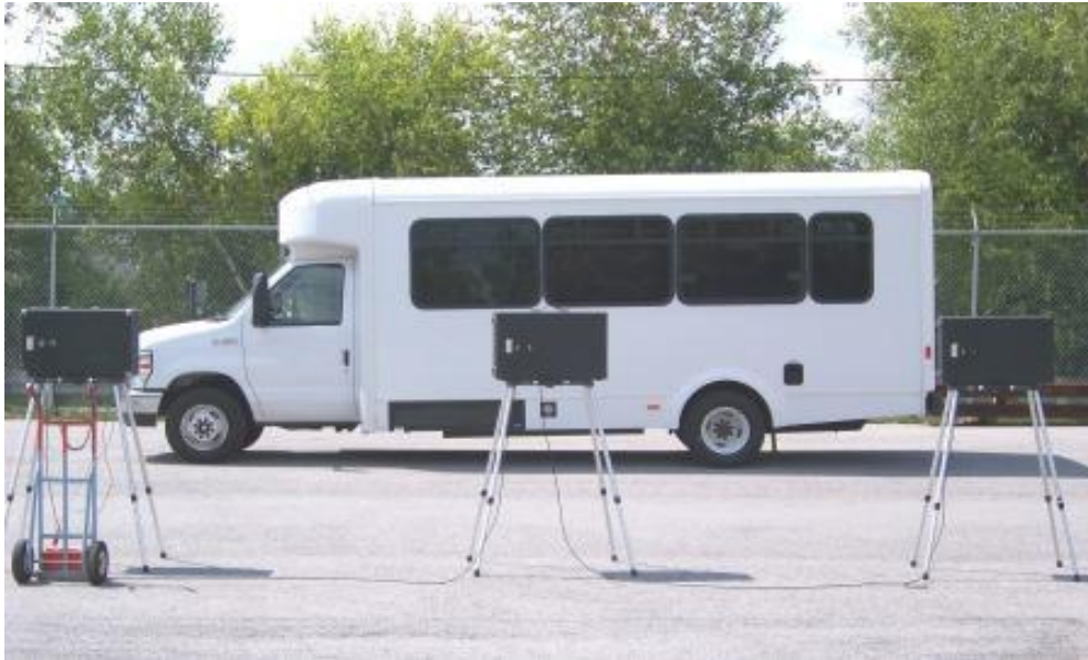
TEST BUS SET-UP FOR 80 dB(A) INTERIOR NOISE TEST
