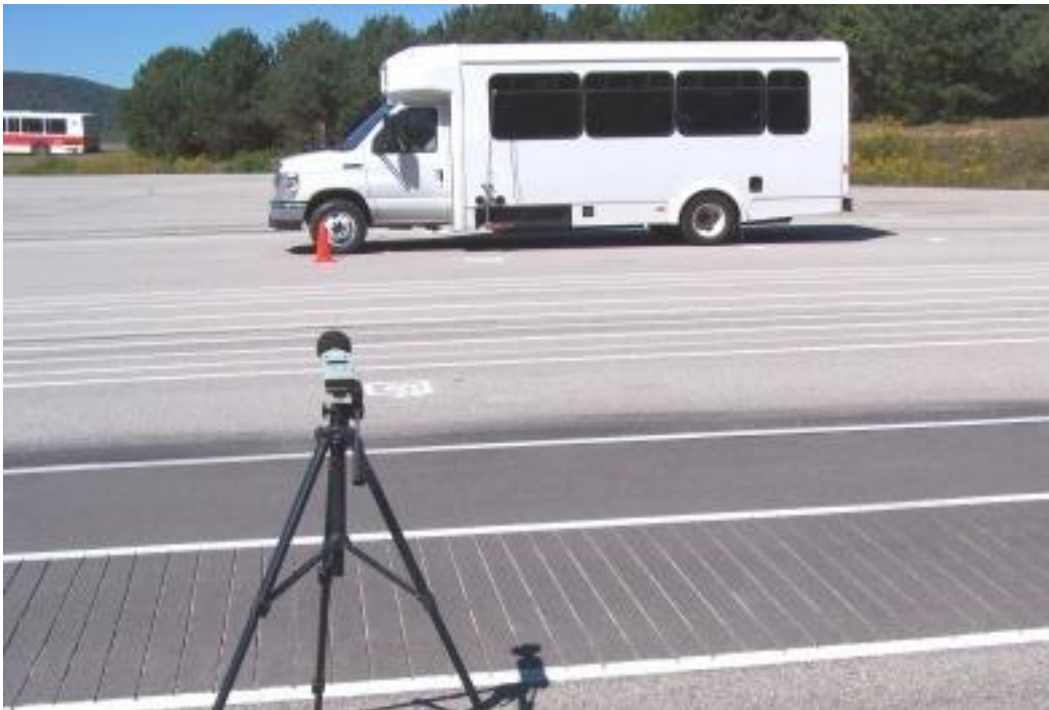
TEST BUS UNDERGOING EXTERIOR NOISE TESTING
