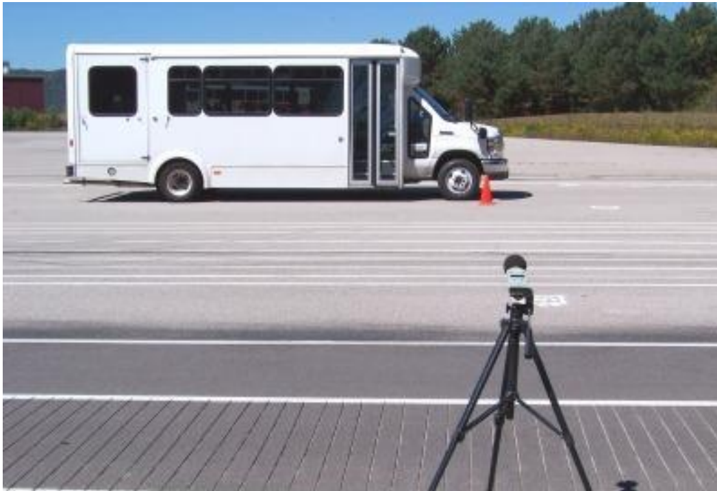
TEST BUS UNDERGOING EXTERIOR NOISE TESTING
