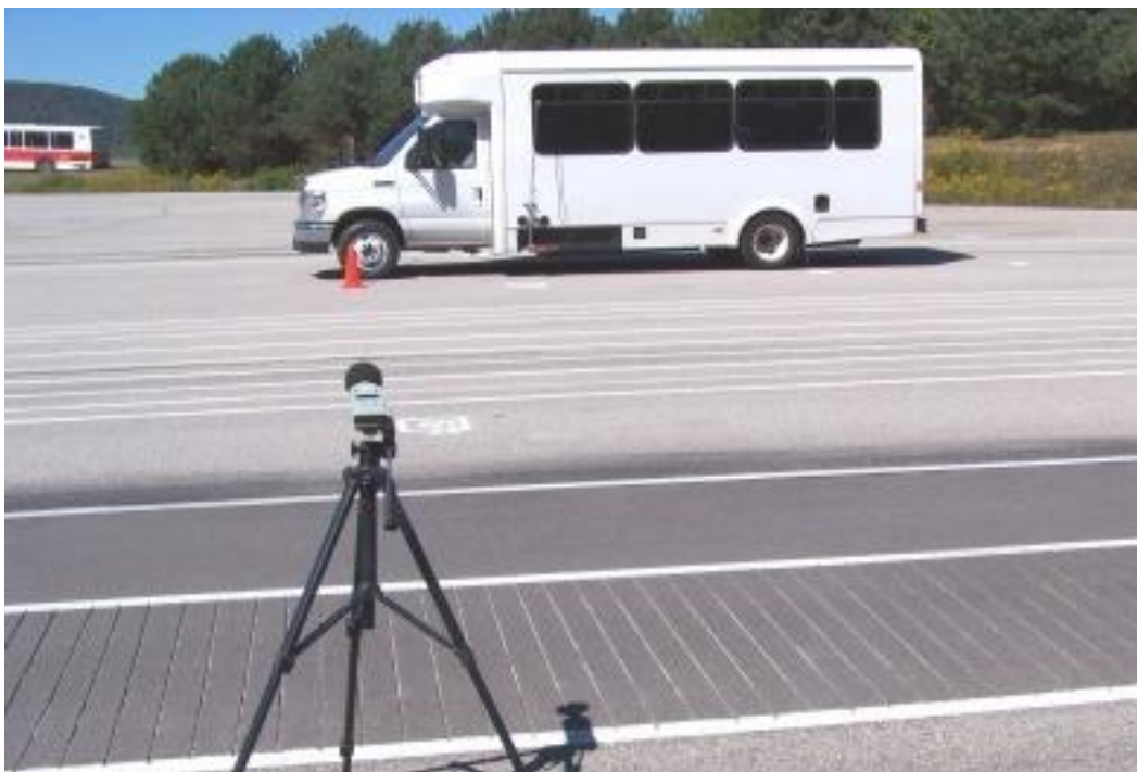
TEST BUS UNDERGOING EXTERIOR NOISE TESTING
