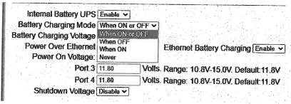
4.1.1.41 The integrated charger must be capable of charging from PoE input with user configurability to enable/disable this featur
