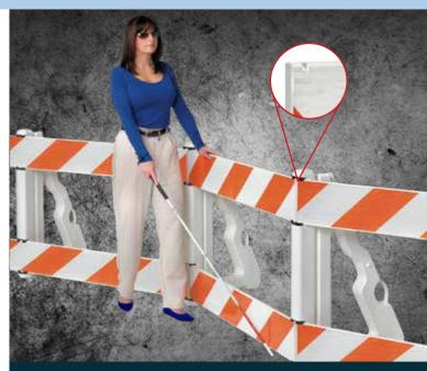
SafetyRail is designed for use with PSS Wave<sup>®</sup> Guide Rail. Upper Rail is smooth, continuous, and safer for the hand. Lower Wave Guiderail measures 1.5" from the ground which reduces potential for trapped cane tips. Wave "Notch" design (see insert) keeps guide rails securely in bushings.
