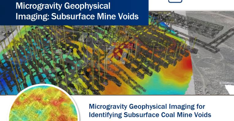
Our proprietary highresolution microgravity imaging provides unparalleled imaging of subsurface conditions, which means more accurate site characterizations. better understanding of risk, more precise remediation targets, and more accurate estimates of remediation costs.
