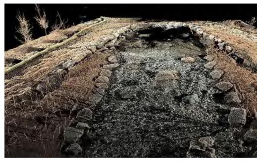
3D As-Built Scan of a Cross Vane
