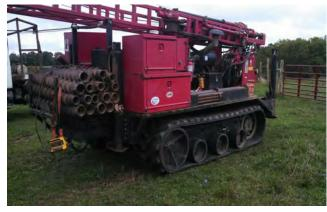
Diedrich D-50 Rubber Track Mounted Drill Rig
