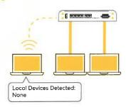
Peplink devices are capable of creating networks where guest users can only see the Internet. This means complete isolation from any other device connected to the router. Also, any devices on the great network will be unable to access the router's WebUI
