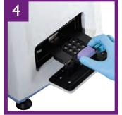
Biochip carrier loaded into Evidence Investigator
