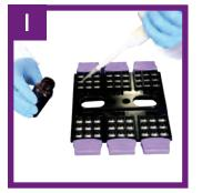
Addition of assay reagents and sample to the biochips
