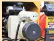
Direct Drive Air Compressor
