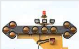
Full Light Kit with Work Area Lighting, Strobe Light, and optional Arrowboard
