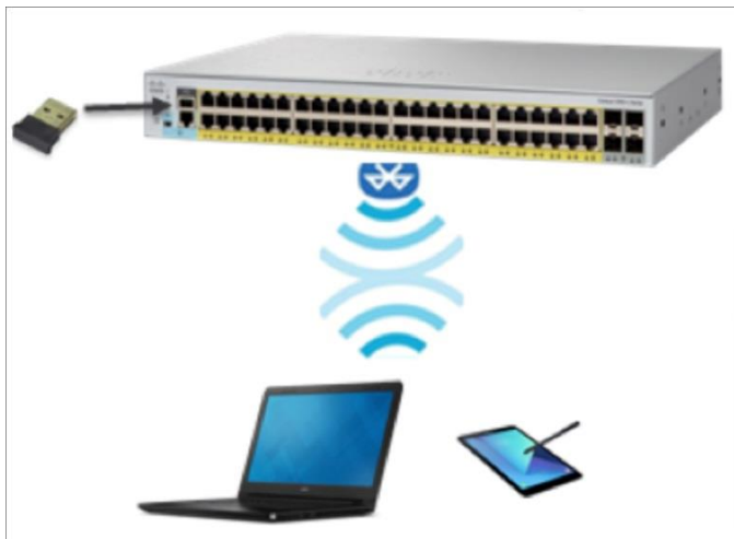
Figure 2. Over-the-air switch access using Bluetooth
