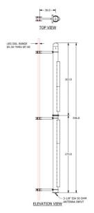
Antenna shown is an RF Channel 7 (174 MHz to 180 Antenna shown is an RF Channel 7 (174 MHz to 180 MHz) High Band VHF Television Antenna. It is shown using the standard mounting brackets supplied with the antenna. Dimensions shown are inches.
