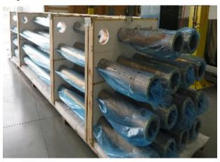
CORTEC Corrosion Inhibitor Impregnated Packing Sleeves
