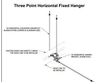
This configuration requires two (2) RLA000-01ALL Universal Horizontal Hanger Bracket and three (3) RLA000-01THRD Horizontal Clevis/Rod Hanger Kit. The horizontal hanger spacing should be an average of every 120-inches (3,048mm) for all rigid line sizes and types. When this configuration is used the RLA000-01HLB Horizontal Lateral Brace to prevent lateral motion is not required. NOTE: Horizontal fixed hangers should only be installed beyond the minimum horizontal run length (see table page 88).
