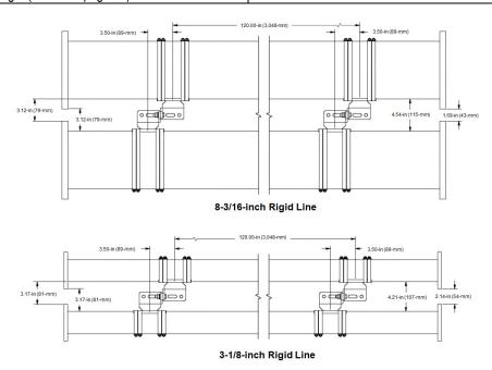
RLA000-01ALL Horizontal Hanger Brackets configured to support two transmission lines side by side.
