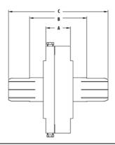
Gas barrier, both sides have at least one pressure port, except the RLA150-16 which has a single pressure port. The assembly has fixed male inner connectors both ends. Includes flange hardware kit.
