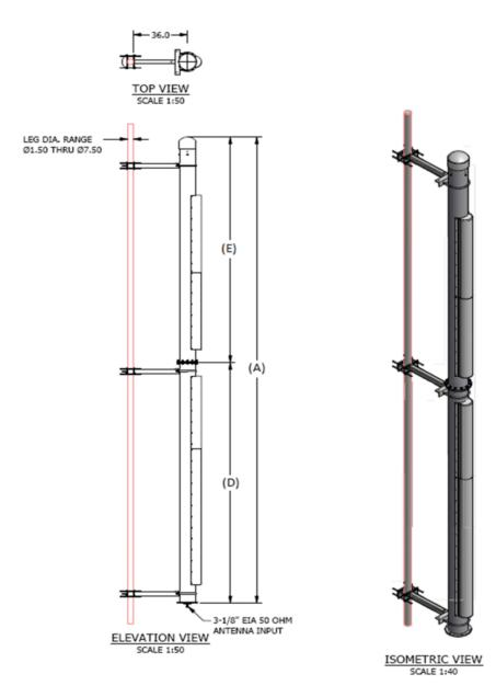
ALV Series VHF television antennas are shipped with 36-inch (914 mm) stand off brackets for mounting on poles or tower legs from 1.5-inches (35 mm) to 7.5-inches (191 mm) OD. Stand off support pipes, face mount brackets, and mounts for larger diameter poles are available from ERI as optional items. Please contact ERI for a proposal for these requirements.
