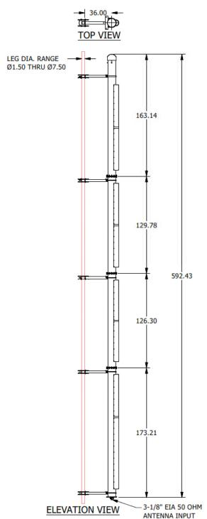
MHz) Model ALV4V7-HSOC-7. Four (4) Bay, Omnioid, Model ALV8V7-HSOC-7. Eight (8) Bay, Omnioid, High Band VHF Television Antenna. It is shown using the standard mounting brackets supplied with the antenna. Dimensions shown are inches.
