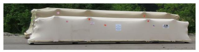
Heat Shrink Skid Tarps Provide Long Term Weather Protection
