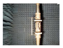
Measurement of antenna patterns on a far-field test range, in a near-field environment, or in an anechoic chamber has been studied and standardized. The correlation between measurements made in the far-field and those made in an anechoic chamber is also an active field of study. Independent radiation pattern measurements of two UHF broadcast antenna arrays are compared and discussed.
