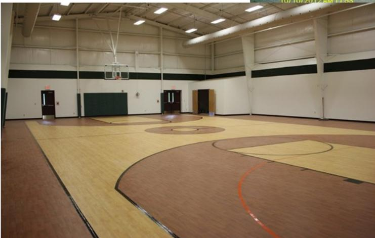
The majority of the structure consists of a pre-engineered metal building, with the entrance being constructed using conventional stick-framed construction.
