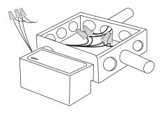
Line voltage wiring connection should be made inside of junction box.
