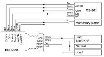
NOTE: Each IR-TEC PPU-300/301 power pack can supply power for up to 6 OS-361 sensors. When more sensors are connected, multiple power packs may be required.
