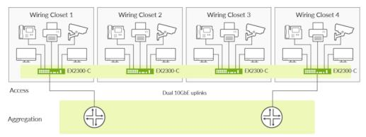
Figure 2: When deployed in a Virtual Chassis configuration, up to four EX2300-C switches can operate as a single, logical device.
