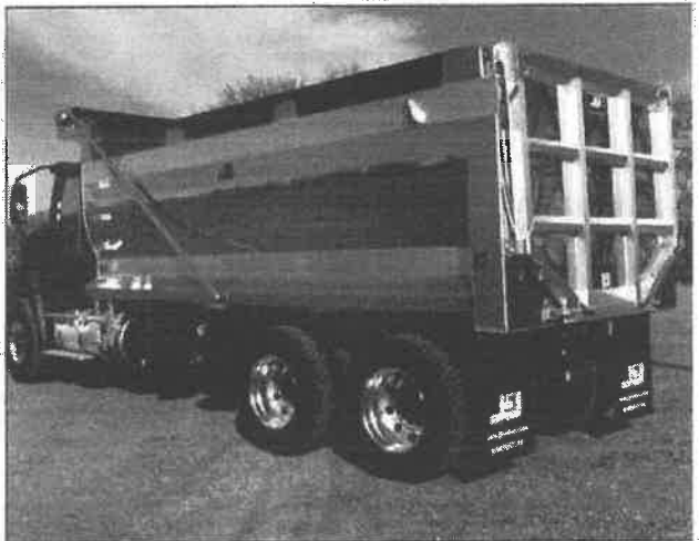
Half round dump bodies are an excellent choice for road paving and maintenance applications.
