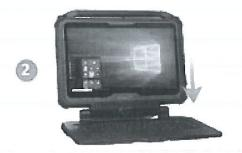
Install the Tablet directly onto the Keyboard docking port, making sure to align the port connectors. The Keyboard and Tablet will automatically function together.
