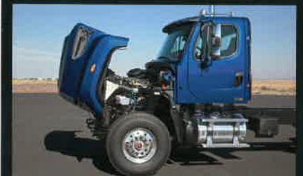
Full tilt hood for easy engine access.
