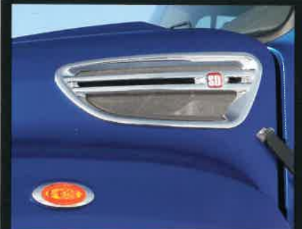
Engine air intake with pre-cleaner for dusty environments.
