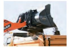
With a sloped bottom for maximum filling and material retention, this is the perfect bucket for day-to-day material handling. Capacities range from 4 to 6.5 yd<sup>3</sup>.
