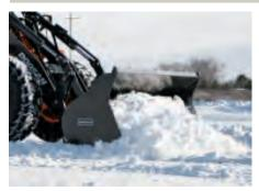
When you need to move snow, mulch or other light material in a hurry, the light material bucket is the economical choice. Comes standard with bolt-on cutting edge.
