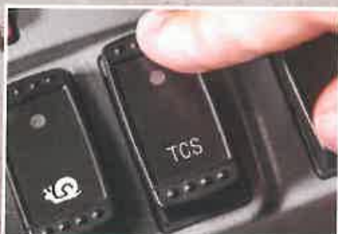
The traction control system reduces tire slippage in wet or wintry conditions.
