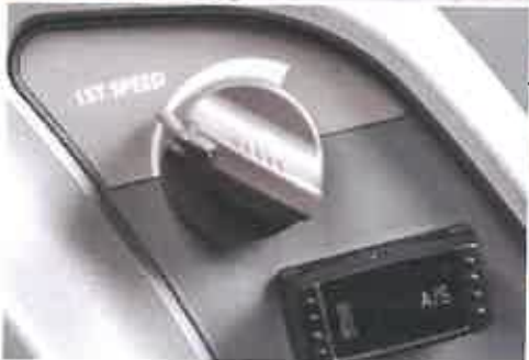
1st speed select switch optimize performance on different job sites.
