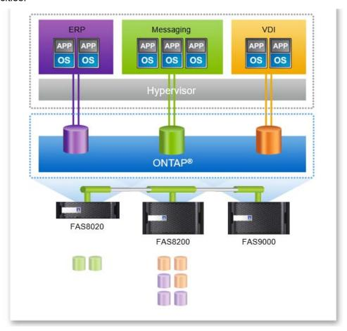
**Figure 4:** Nondisruptive operations – Move data to available nodes and retire existing hardware.
