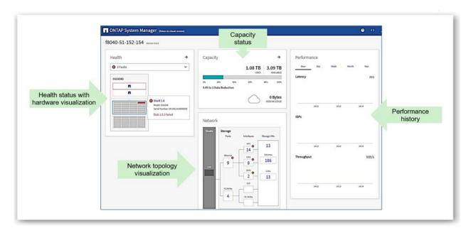
**Figure 7: Intuitive ONTAP System Manager** —Based on REST APIs, the new System Manager dashboard is more intuitive and displays richer information in a more actionable view.
