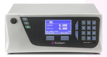
The Serinus<sup>®</sup> 50T Trace Sulfur Dioxide  $(SO_2)$  analyser delivers precise and reliable performance at excellent value. It uses proven pulsed UV fluorescent radiation technology to measure  $SO_2$  in ambient air (LDL 100 ppt, range 0 - 2000 ppb).
