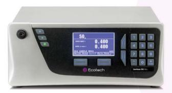
The Serinus<sup>®</sup> 50 sulfur dioxide (SO<sub>2</sub>) analyser delivers precise and reliable performance at excellent value. It uses proven pulsed UV fluorescent radiation technology to measure SO<sub>2</sub> in ambient air (LDL < 0.3 ppb, range 0 to 20 ppm).
