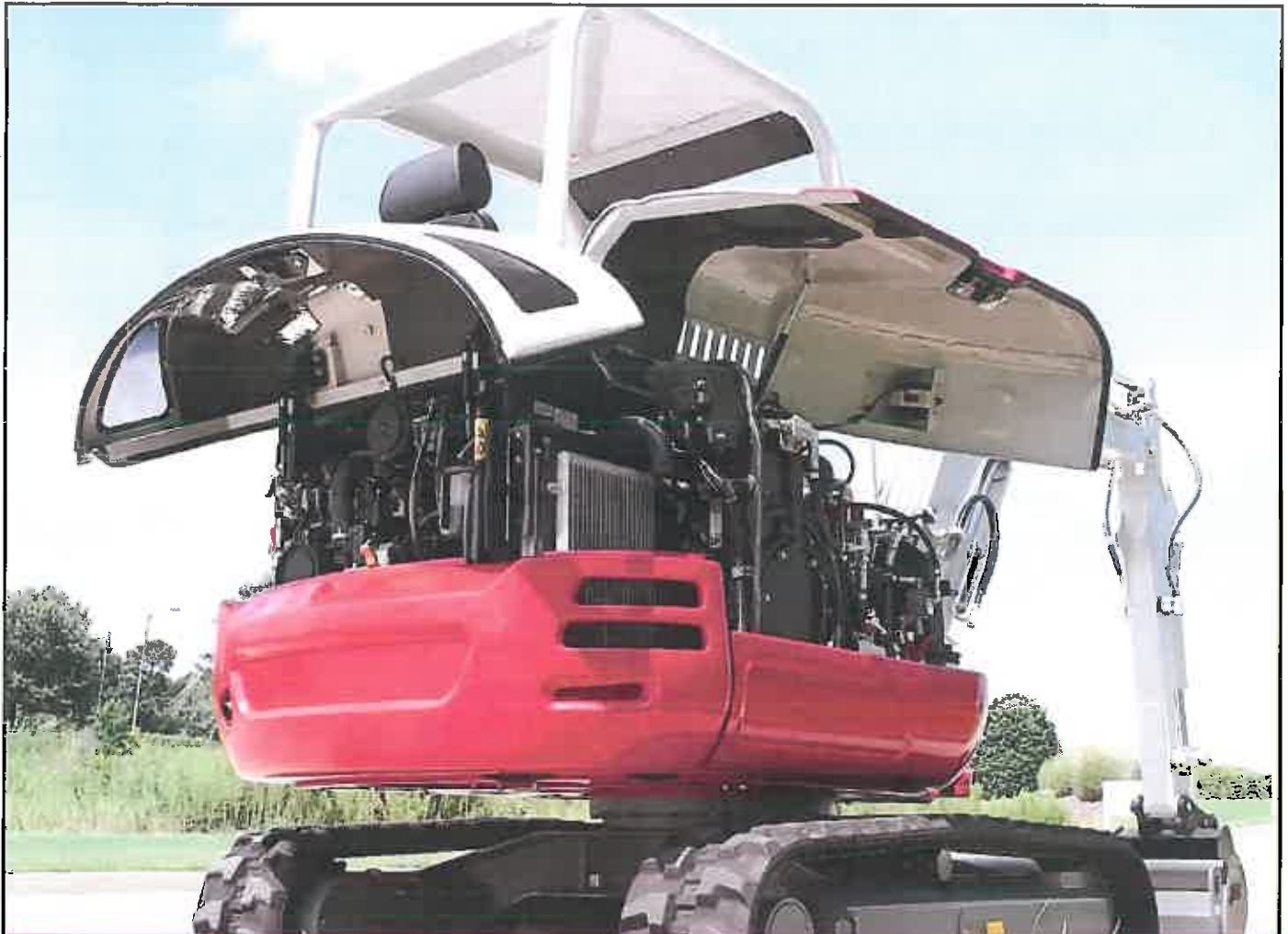
Lockable service hoods lift overhead for outstanding maintenance access.
